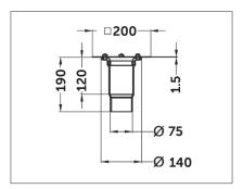
For a fast and vapour sealed installation of the Akasison XL75 in metal roofs and for pre-completion building drainage when insulation and roof outlets are not yet installed. Includes a small metal plate and HDPE connection pipe.
